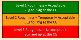
Using aircraft simulation, APR can predict the CG's response to the runway's measured profile and determine if the roughness is acceptable, excessive or unacceptable using Boeing's criteria. APR's technology, called **BBI+**, can overcome the limitations of BBI and still provide you with the guidance developed by Boeing and approved by the FAA.
